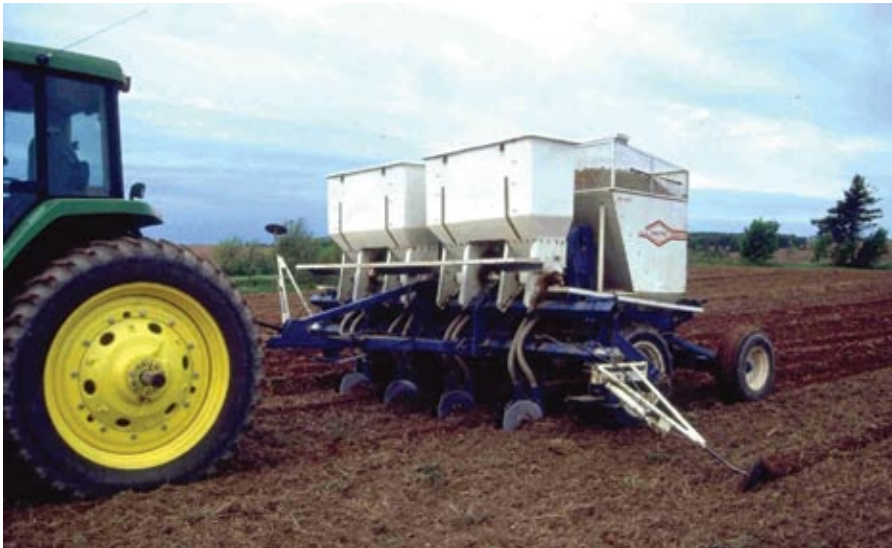
Figure 7: Planting Potatoes into 25 to 30 % Crop Residue
